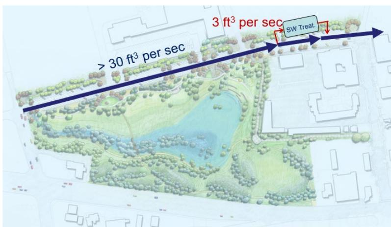
In the Fall of 2010, the City completed the Legacy Park project. The Legacy Park project included the construction of a new 8 ac-foot (350,000 cubic feet) storm water detention basin, an irrigation system, and the planting of native plants and trees. The addition of this storm water detention basin along with the Civic Center Storm Water Treatment Facility provides 100% compliance with the water quality standards for Malibu Creek and Lagoon.
